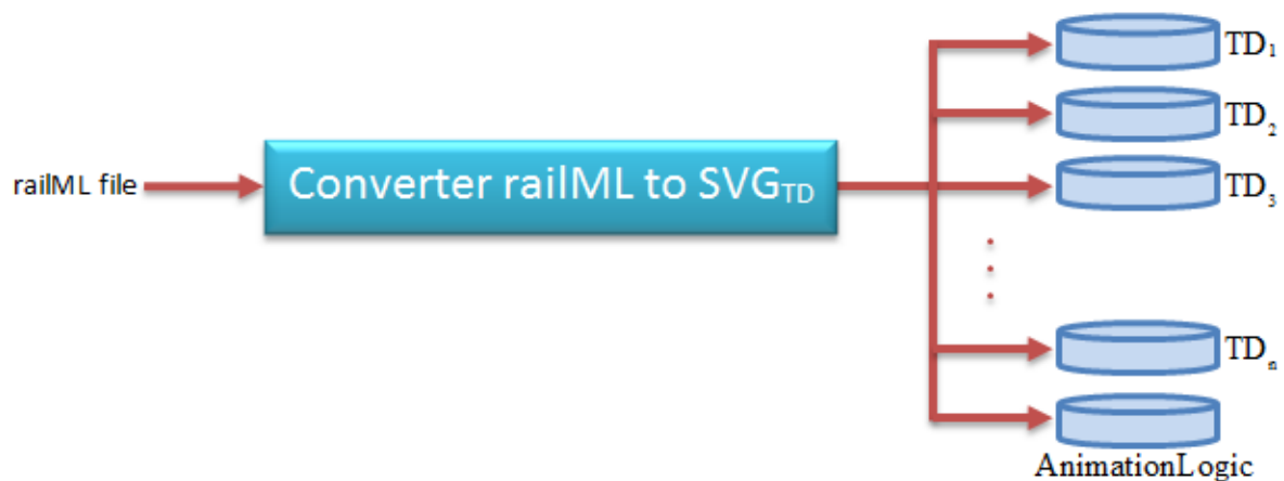
Figure 2 - RailML to svg conversion process
